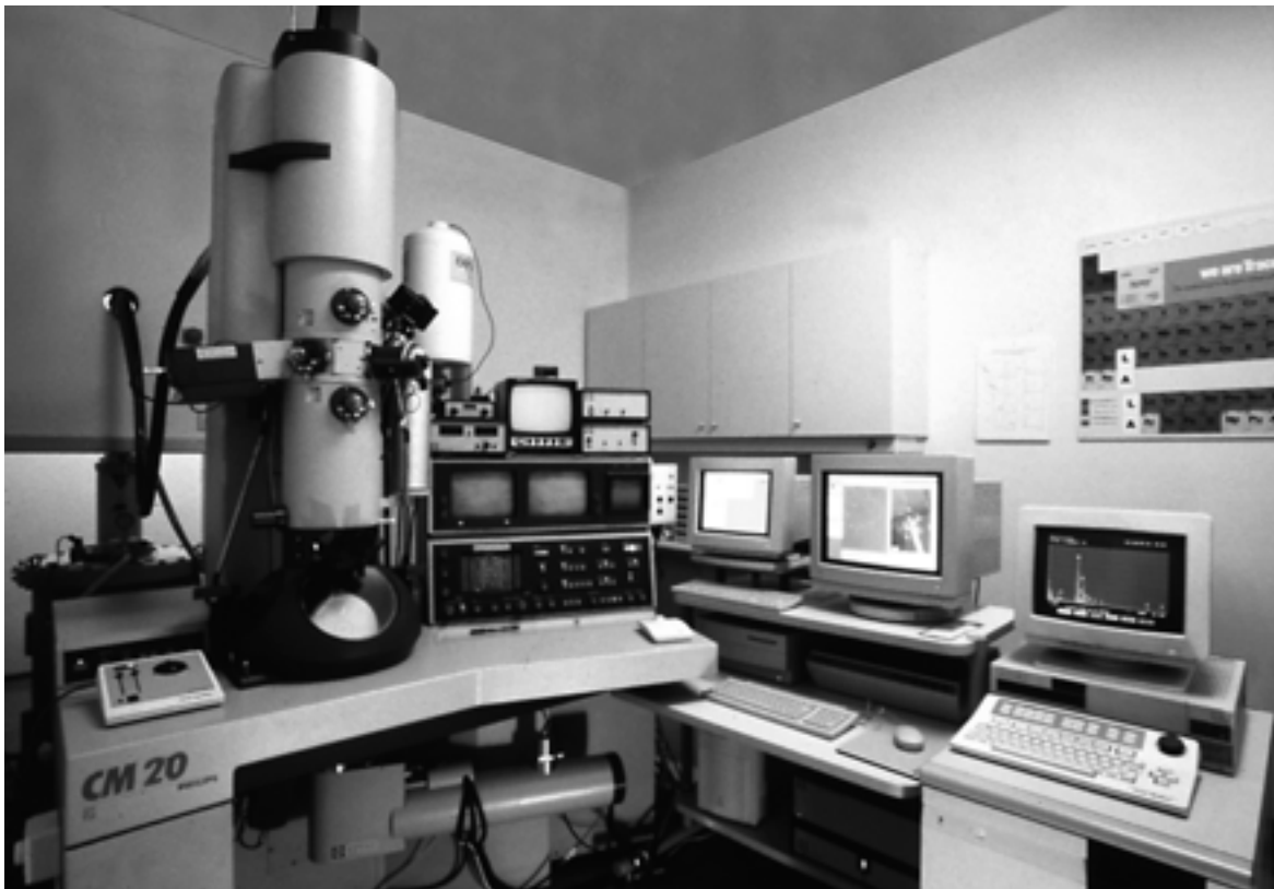
Philips CM20 TEM/STEM with twin lens, LaB 6 cathode, with a Gatan Imaging Filter and Noran HPGc EDX spectrometer (installed from 1989-1994)
