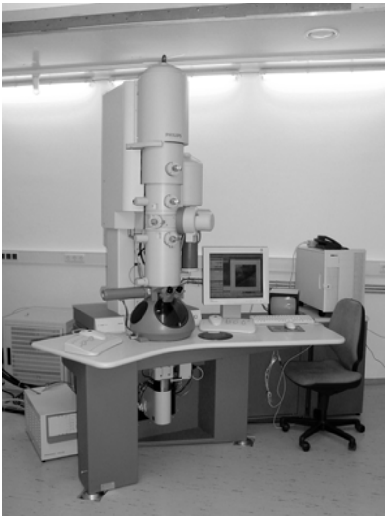
December 2000: The Tecnai F20 already installed in the institute (in the room shown above)
