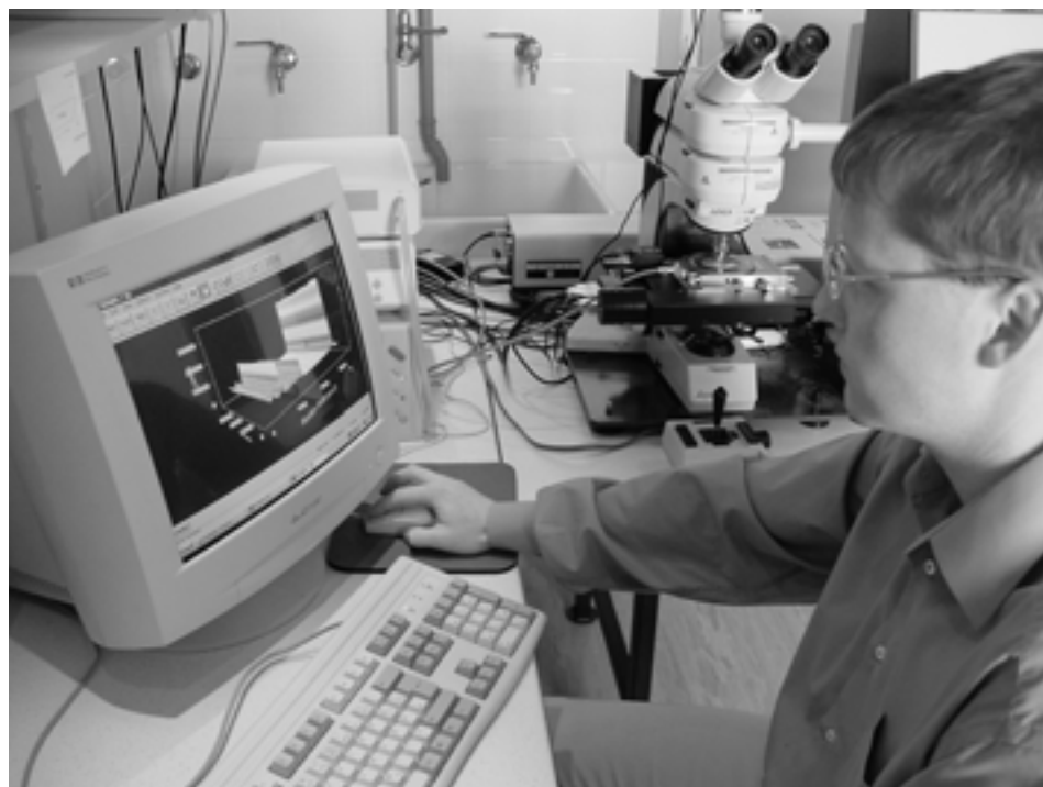
Raman microscope: Renishaw 2000 With a LEICA research microscope and a dual laser system: diode laser (782 nm) & HeNe laser (633 nm)
