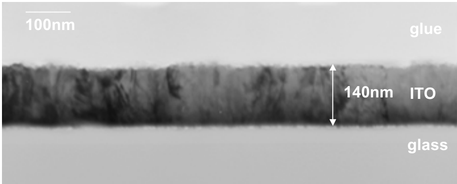
Fig.1a TEM bright-field image of an unetched ITO layer
