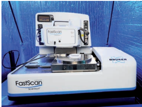
AFM Bruker FastScan Bio In situ atomic force microscope with PeakForce probes
