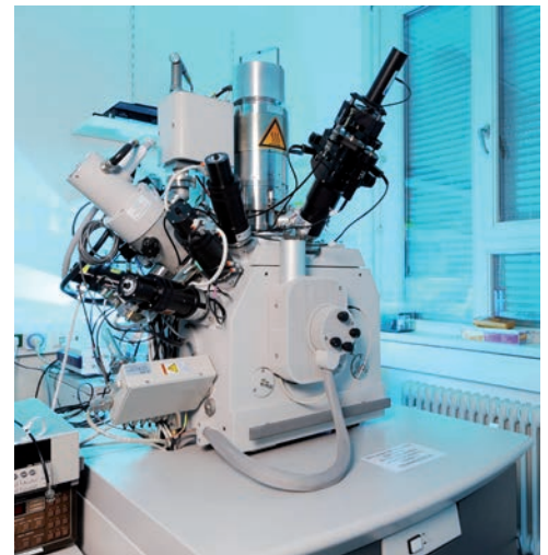
Focused Ion Beam FEI Nova 200 DualBeam FIB-SEM, FEG and Ga-ion source, Omniprobe manipulator, various gas injection systems, XFlash X-ray spectrometer (Bruker), AFM in situ SEM (GETec)
