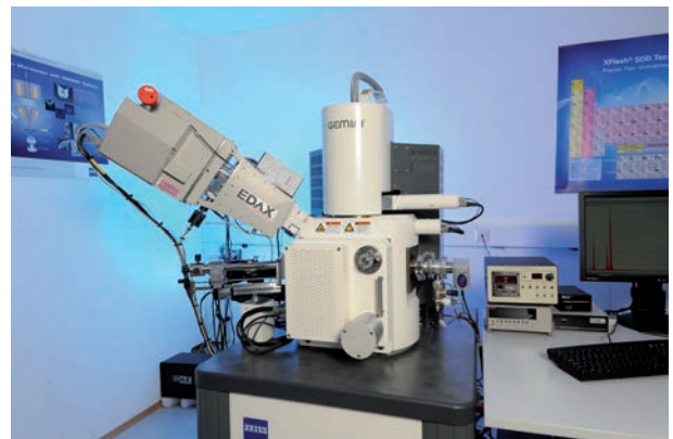
HR-SEM ZEISS Ultra 55 Analytical high resolution SEM, FEG, STEM-, EsB-, AsB- and in-lens detectors, EDX- and WDX-spectrometers (EDAX), EBSD-detector (EDAX), heating stage up to 1050°C (Kammrath & Weiss)
