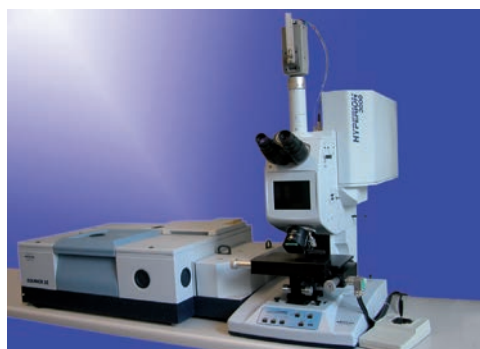
Bruker FT-IR microscope Infrared microscope Hyperion 3000 with Tensor 27 spectrometer, ATR and GIR objective, FPA and MCT detectors
