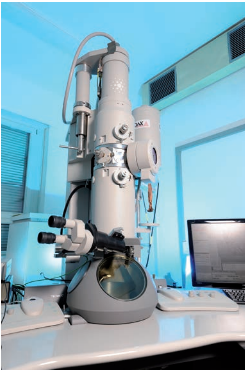
Bio-TEM FEI Tecnai12 Transmission electron microscope, LaB6, 120 kV, low-dose CCD (Gatan), cryo-transfer system (Gatan) and Freeze plunger (Leica)
