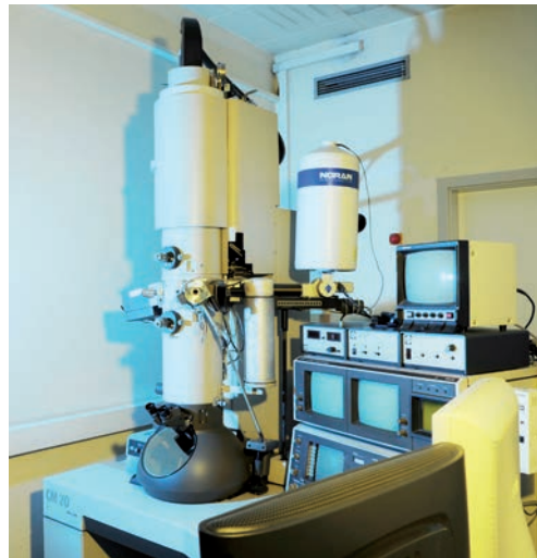
TEM Philips CM20 Analytical TEM, LaB6, STEM, EDX-spectrometer (Noran) and Imaging Filter (Gatan)
