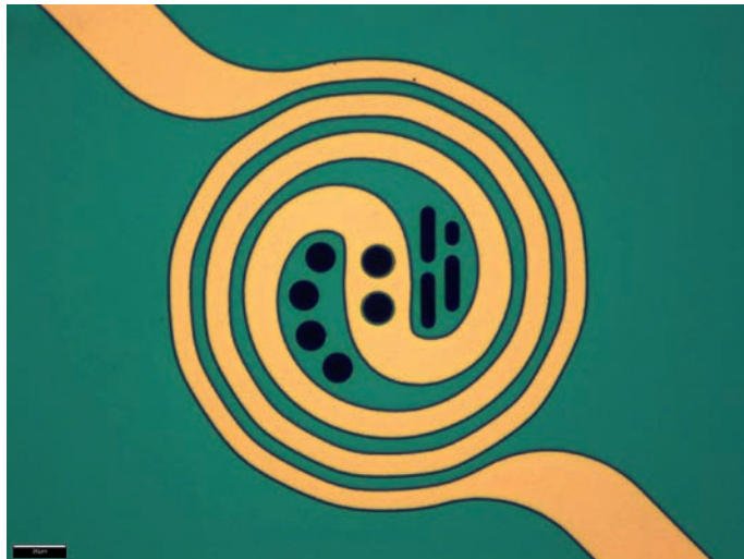
Figure 2: DENStolutions Wildfire™ S3 nano-heater, resistively heated metallic spiral layer with a diameter of approx. 150 μm. Light microscopy image (Alicona IFM).
