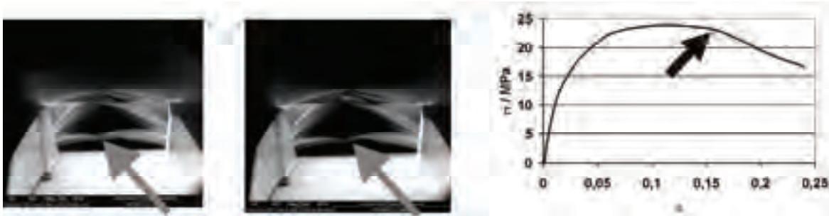
Fig.1 Images cut out from a video to the left (left) and the right (center) of the kink marked by an arrow in the corresponding stress-strain diagram (right); image width: 6.2 mm.
